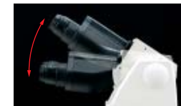
Tilt angle is adjustable 8°–32°.
